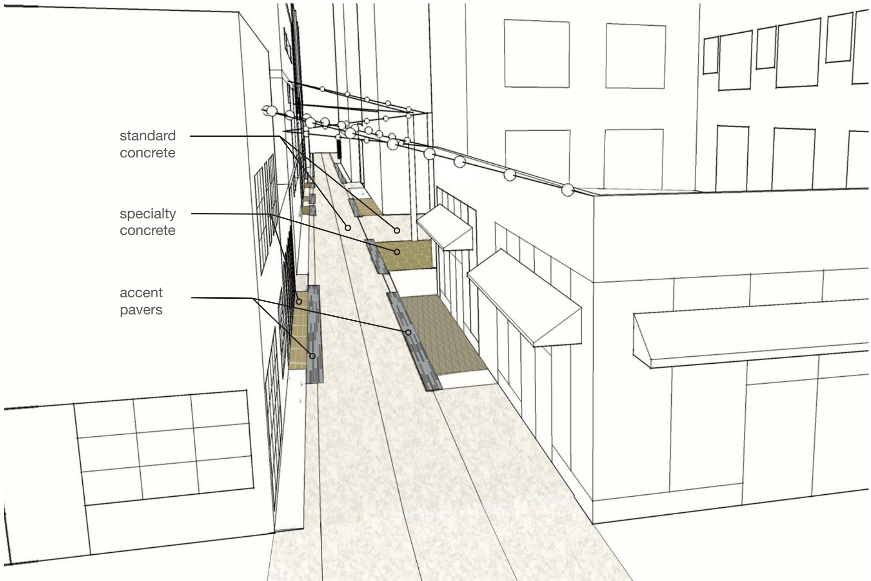
Figure 14: A diagrammatic illustration of where various pavement types should appear within the alley.
