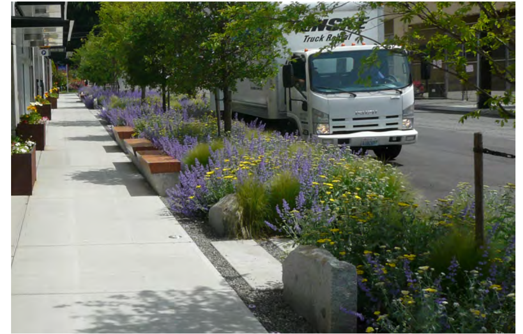
A generous understory of plantings is recommended for all green streets. These add visual interest along the sidewalk, reduce impervious area and runoff, provide habitat and provide a buffer between pedestrian areas and vehicles.
